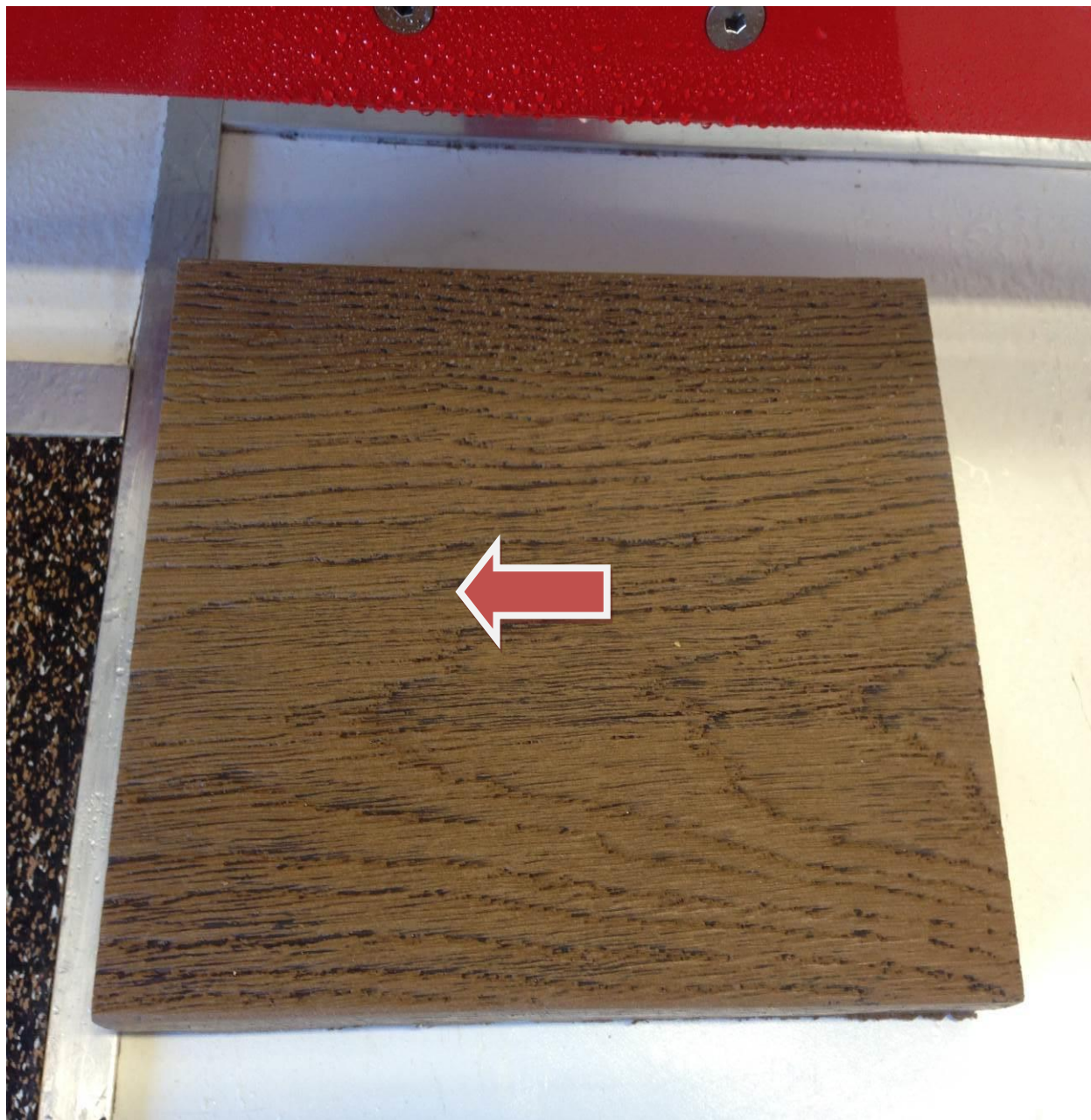
Figure 1: Millboard Composite timber. Arrow indicates direction of test.
